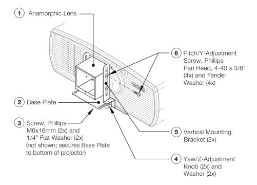
Figure 3-19. Prismatic Anamorphic Lens Mounting Assembly - Exploded View
